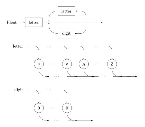
The identifiers constructed this way can be recognized by the following finite automaton:
