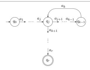
Let  $u = a_1 \dots a_j$ ,  $v = a_{j+1} \dots a_k$ ,  $w = a_{k+1} \dots a_r$ . Then according to the properties of j and k it holds that  $v \neq \varepsilon$  and  $|uv| \leq n$ . Besides, it is clear that the automaton  $\mathcal{A}$ , while recognizing, can go through the  $q_j$ -loop any number of times, i. e., for all  $i \in \mathbb{N}$  it holds that:  $uv^i w \in L$ .  $\Box$
