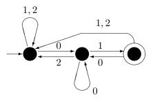
The number of states of this DFA can not be further minimized. There are examples, where the DFA given in the proof of the RABIN-SCOTT theorem cannot be further simplified, i.e., if the given NFA has n states, then in the worst case the DFA actually needs  $2^n$  states.
