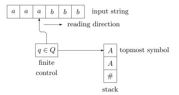
3.1 **Definition (push-down automaton)**: A (*nondeterministic*) *push-down automaton*, shortly PDA, is a 7-tuple
