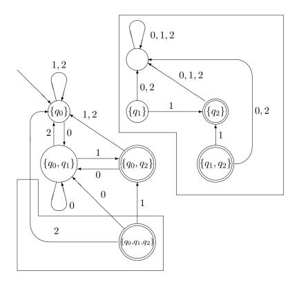
The fragments in boxes  $\Box$  are unreachable from the initial state  $\{q_0\}$  of  $\mathcal{A}_{01}$ . Therefore,  $\mathcal{A}_{01}$  can be simplified to the following equivalent DFA :
