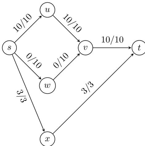
In the lecture we have seen that given a maximum flow, one can compute a minimum  $s$ - $t$  cut  $(A^*, V \setminus A^*)$ , where  $A^*$  is the set of nodes that can be reached from  $s$  on a path with positive residual capacities in the residual graph. Give the cut  $(A^*, V \setminus A^*)$  in  $G$ . (3 Points)
